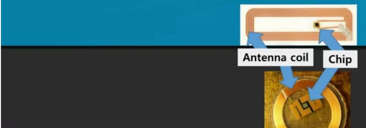
The diagram shows a top-down view of a rectangular RFID tag with a copper-colored antenna coil and a small black chip. Below it is a circular gold-colored tag with a similar antenna coil and chip. Blue arrows point from the labels 'Antenna coil' and 'Chip' to the respective parts in both images.
